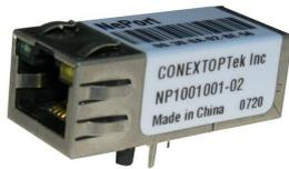
The NPPort is the most compact, integrated solution available to PoE-enable any device with an standard rj45 connector. By simply adding NPPort to a product design, device manufacturers cut their design cycle by as much as 80% and are able to offer PoE Ethernet connectivity in record time.
